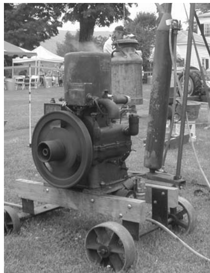
This milk can lifter from the Raymond Maybie Farm can easily heft 100-pound milk cans.
