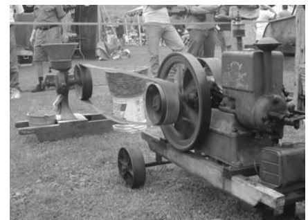
This corn grinder takes the individual kernels of shelled corn from the machine pictured above, and crushes it to make cracked corn for livestock.
