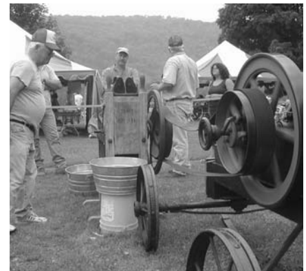
Ears of dried corn are fed into this corn sheller by my father, and the individual kernels are removed from the ears.
