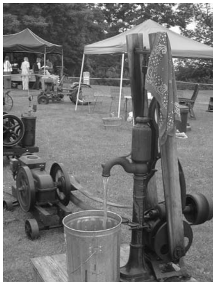
This water pump from the Maybie farm has been adapted to run by belt and could easily water the 125-head dairy herd.
